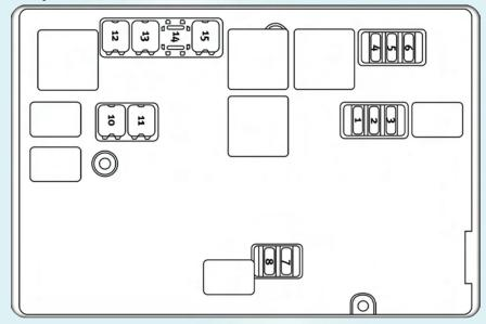
• The Integrated Power Module (IPM) is located in the engine compartment on the right hand side near the Washer Fluid Reservoir. This module contains fuses and relays.
