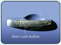
Both front door handles have LOCK buttons located on the outside of the handle, with one of the vehicle's Passive Entry Key Fobs within 5 ft (1.5m) of the driver's or passenger side, press the door handle LOCK button to lock all four doors.
