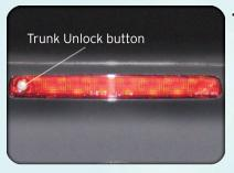
With a valid Passive Entry Key Fob within 3 ft (1.0m) of the deck lid, press the button on the left side of the CHMSL (Center High Mounted Stop Light) which is located on the deck lid.
