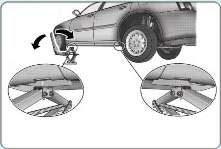
Raise the vehicle by turning the jack screw clockwise. Raise the vehicle only until
